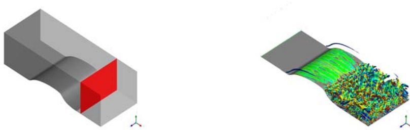
(a) Location of traversing plane behind the hump (b) Visualized vortex structures behind the hump
