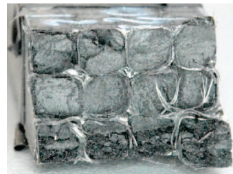
Fig. 2: Fracture area of beam loaded in four-point bending
