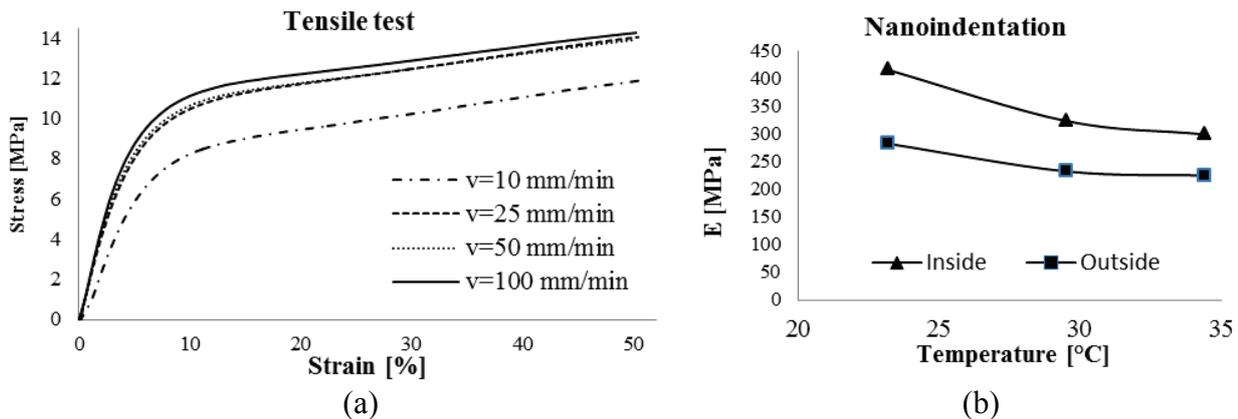
Fig. 1: a) Tensile test stress-strain curve of recycled plastic under different strain rates, b) Evolution of Young's modulus measured by nanoindentation as a function of temperature
