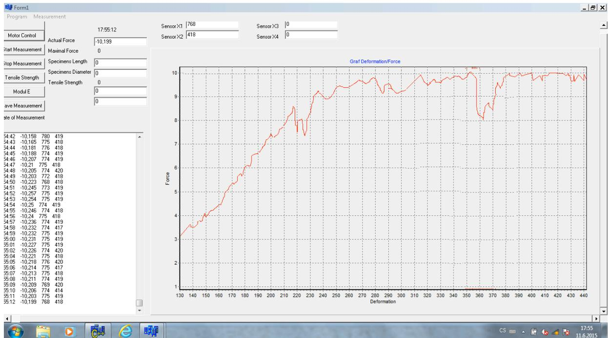
Fig.2 Window of software used for control of portable device and for calculation of material properties. The software draws a graph of the loading forces and deformations.
