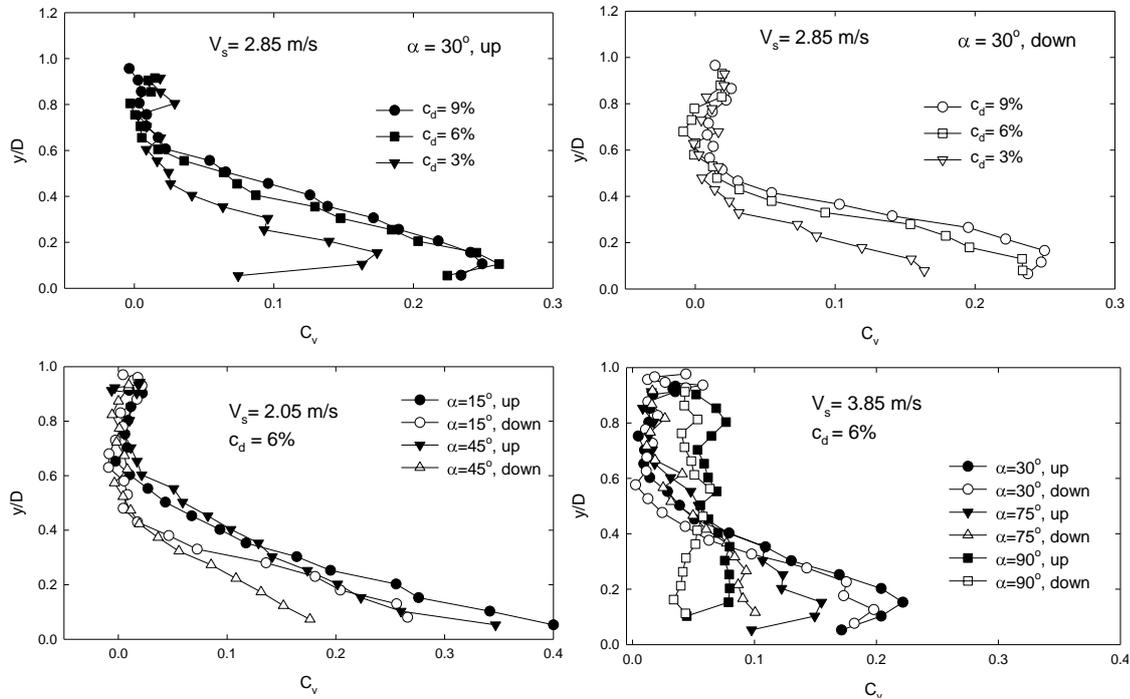
Fig. 2: Effect of the transport concentration  $c_d$  and flow direction on profiles of local concentration  $c_v$ .
