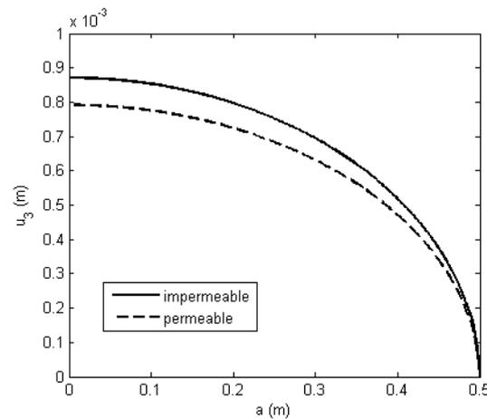
Fig. 1. Influence of the electromagnetic conditions on the crack displacement under a combined load.
