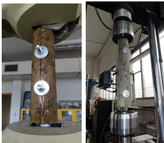
Fig. 1-A/B: Tested sample in the press EU 100 (A - left), dynamic test - Pulsator INSTRON (B - right)
