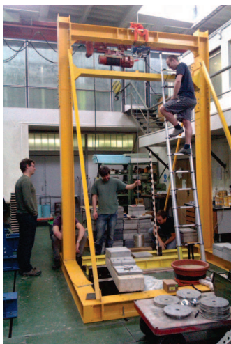
Fig. 1: Steel frame with hoist.
