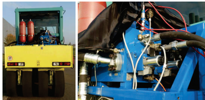
Fig. 1: Energy regeneration module prototype mounted to the vehicle
