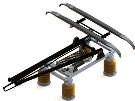
Fig. 1: The author's original concept model of pantograph
