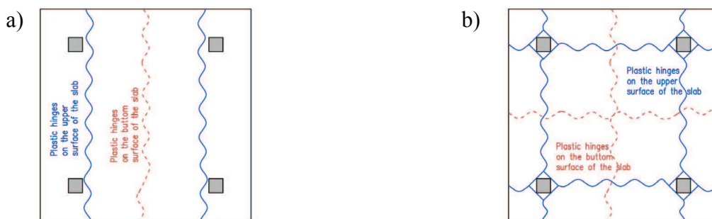
Fig. 1: Patterns of destruction of the internal area of a continuous slab (described in the text)
