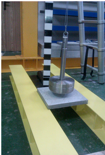
Fig. 1 Specimen supported by beams.
