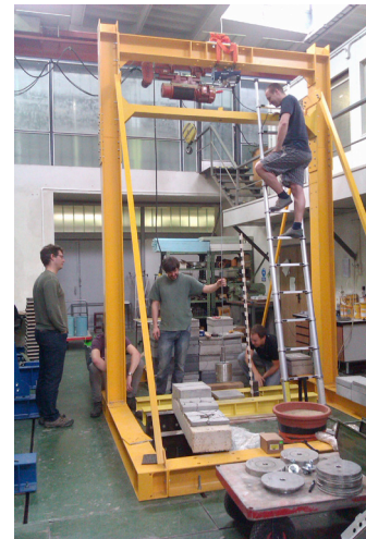
Fig. 3 Steel frame with hoist.
