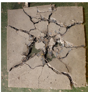
Fig. 10 Radial crack pattern.
