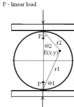
Fig. 3 Brazilian test: parameters  $\theta_1$ ,  $\theta_2$ ,  $r_1$  and  $r_2$ .
