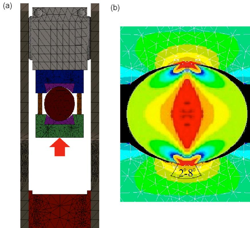
Fig. 5 a) FEM model of portable device; FEM model of contact between jaws and specimen.
