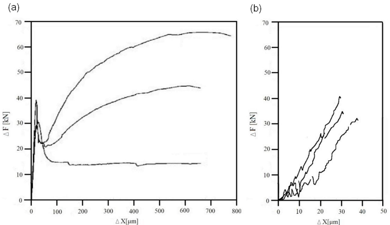
Fig. 4 Experimental graph shows relationships between loading force and measured deformation: a) loading to the final fracture; b) linear region at the beginning of the test.
