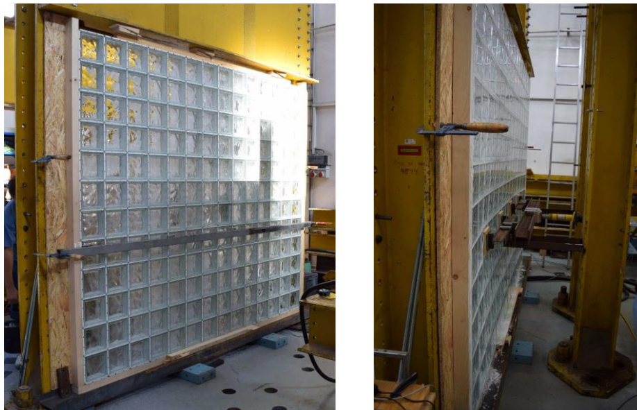
Fig. 3: The completed wall prior to filling of the joints (left) and during the test (right).
