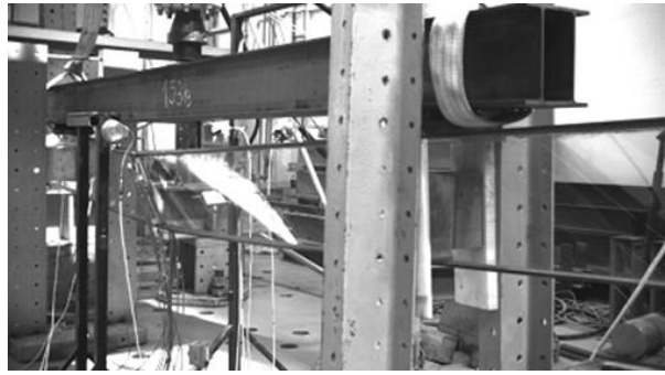
Fig. 1: Buckling of the hybrid steel-glass beam.
