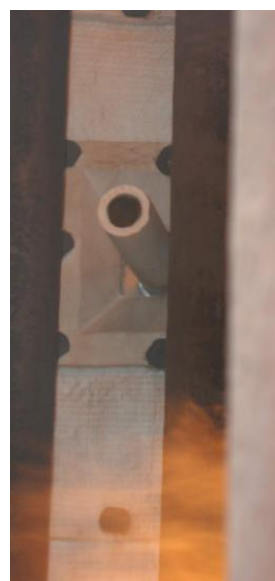
a) Fired heater scheme and observation doors levels. b) Heat flux meter in one observation door.
