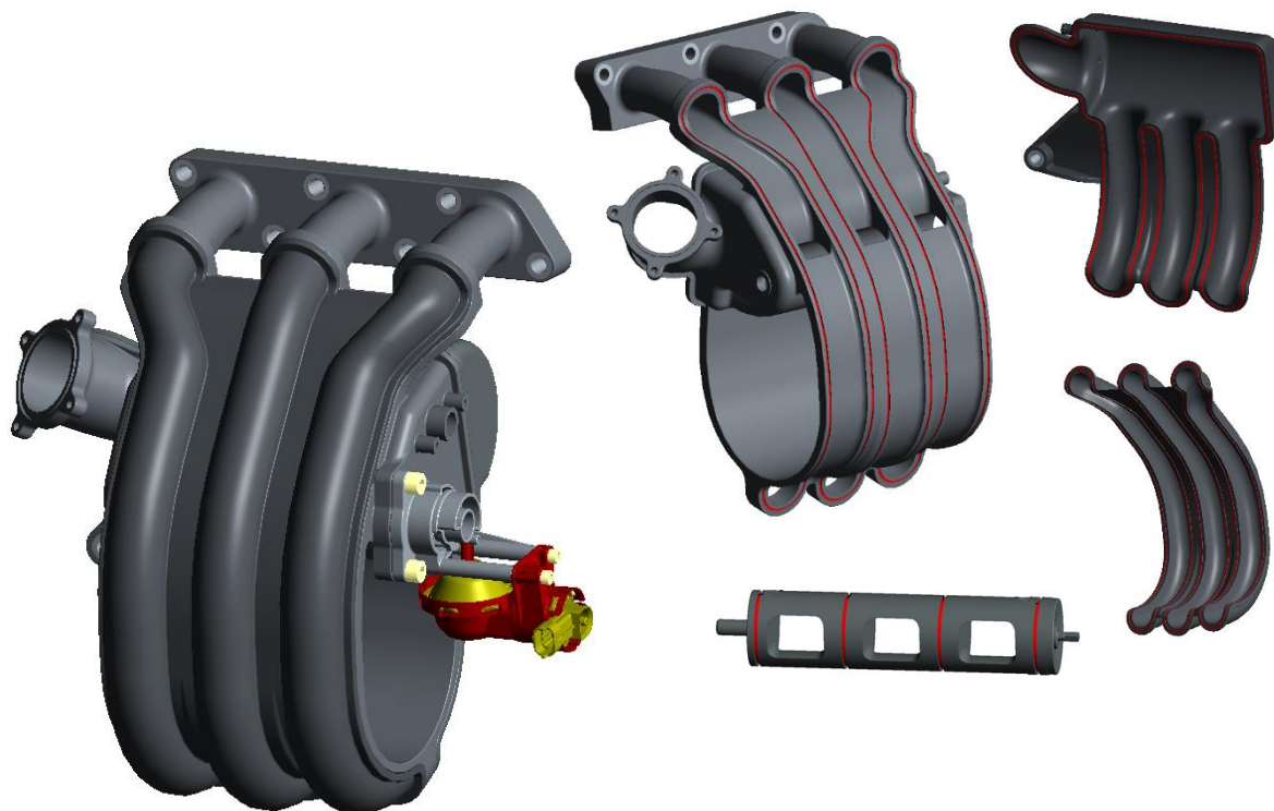
Fig. 5: 3D model of designed variable intake manifold (Reichrt, 2015).
