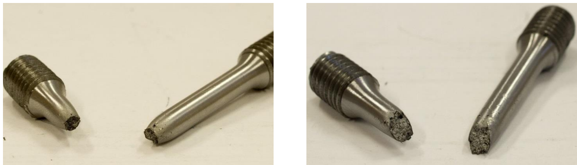
Fig. 6: Fractured samples produced wit parameters a) No. 1; b) No. 2.
