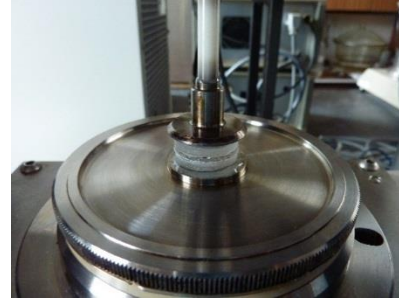
Fig. 4: Specimen glued to rheometer plates.
