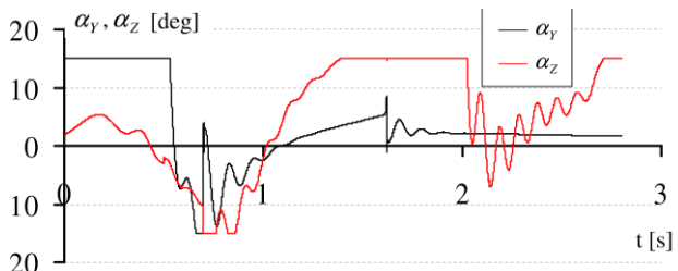
Fig. 5: The realized angles of the flight control in the channel of height and direction for the single executive system.
