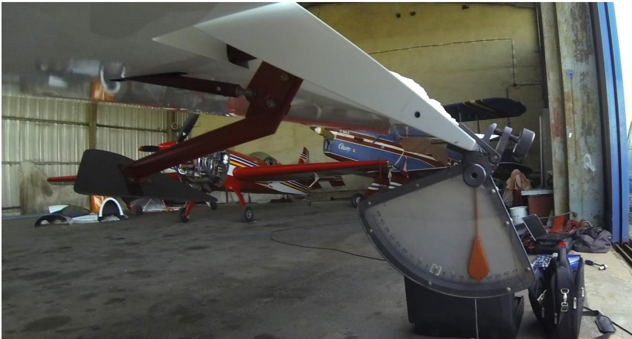
Fig. 4: Calibration of control surface deflection.
