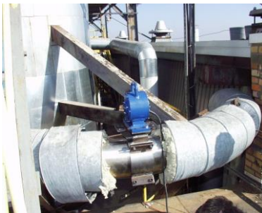
Fig. 5: The method of excitation of the resonant vibrations in the pipeline.
