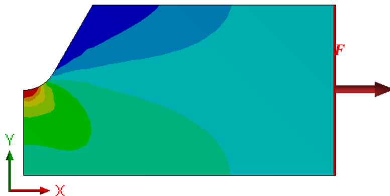
Fig. 3: Stress distribution map for the notched specimen.
