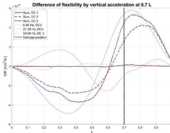
Fig. 3: Differences of flexibility at the midpoint  $0,7L$ , passing velocity  $v = 0.2$  m/s.
