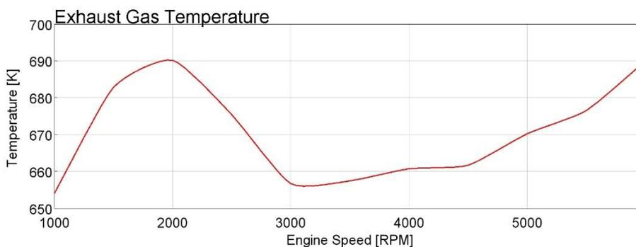
Fig. 4: The exhaust temperature for Case 2.
