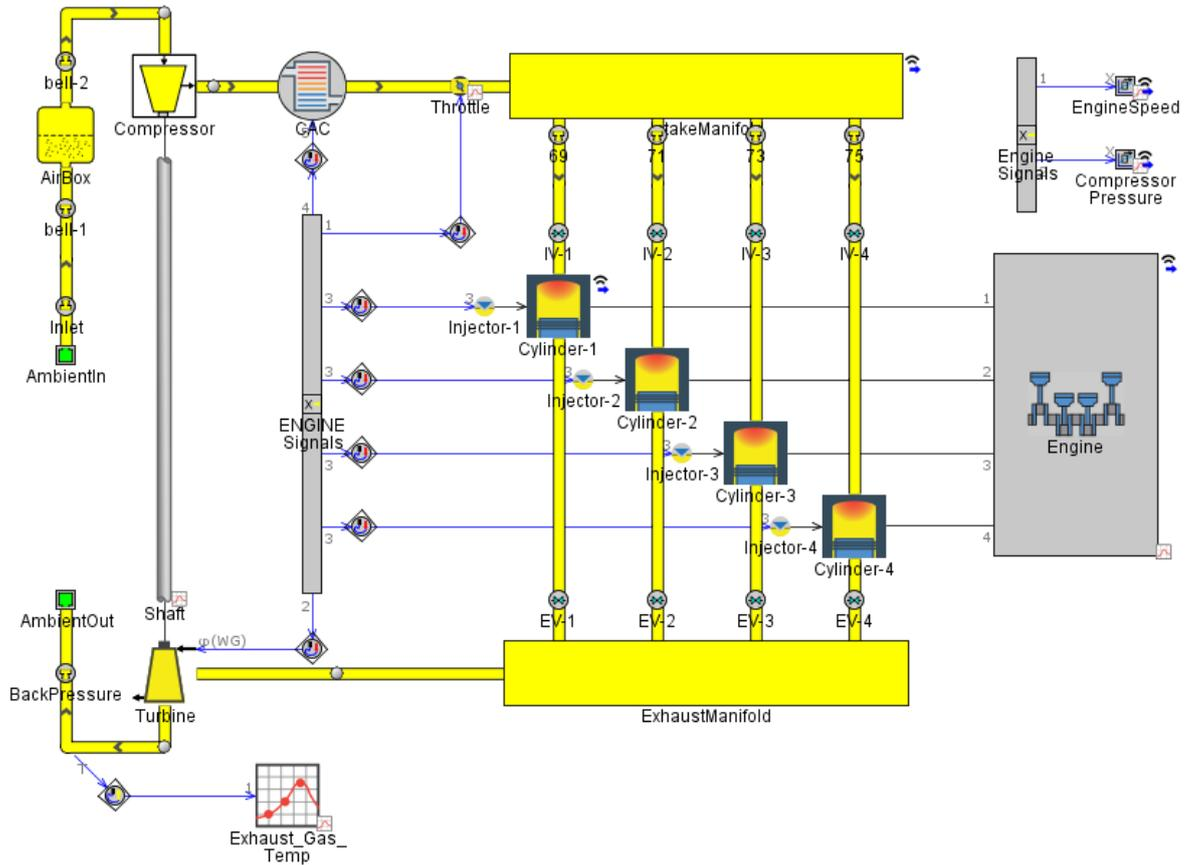
Fig. 1: Engine simulation model.
