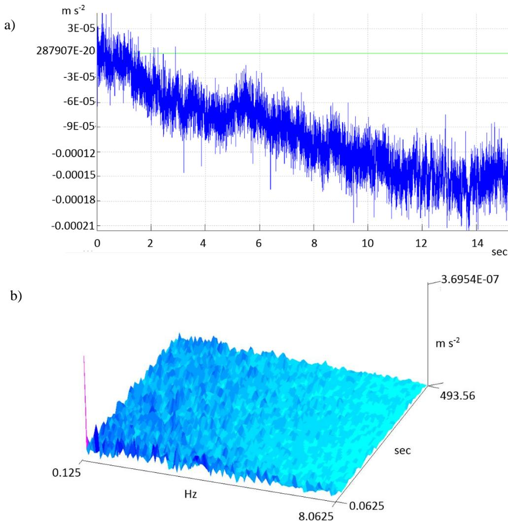
Fig. 3: Graphical interpretation of test results for a point 500 m away from the mast foundation, a) time history, b) signal spectrum.
