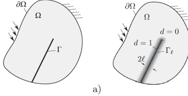
Fig. 1: Fracture region  $\Omega$  with crack surface  $\Gamma$ : a) Sharp example of crack topology; b) arranged example. The crack is described by the phase-field variable  $d = 1$ , whereas  $d = 0$  means undamaged material. The crack is arranged over the length scale  $l$ .
