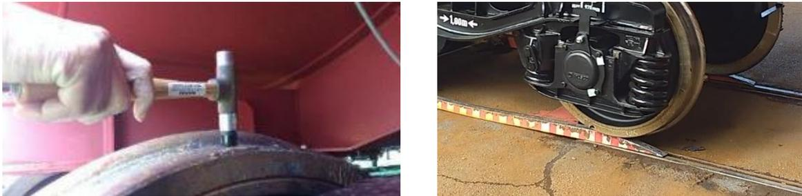
Fig. 1: Applying a modal hammer and gravitational impact.
