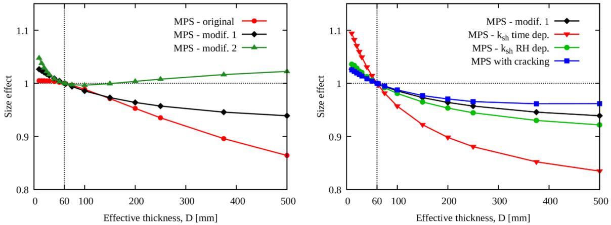
Fig. 2: Size effect on drying shrinkage of prisms of different sizes. Results were obtained with MPS model with different values of parameter  $p$  (left) and with parameter  $p = \infty$  and modified shrinkage relationship or cracking (right).
