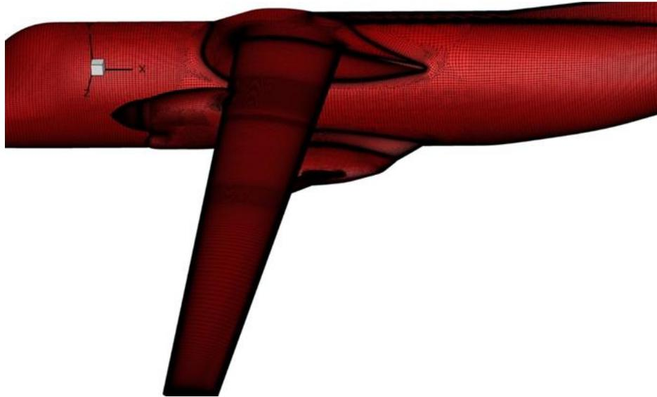
*Fig. 2: Example of surface grid over the computation model. It can be seen that main part of airplane is meshed by hexahedral elements. Using of tetra-elements was necessary in complex geometry regions as wing-fuselage transition or wing-nacelle. Usage of hexahedral elements leads to reduction of volume elements that influence the computation time positively. (Shortened computational time etc.)*
