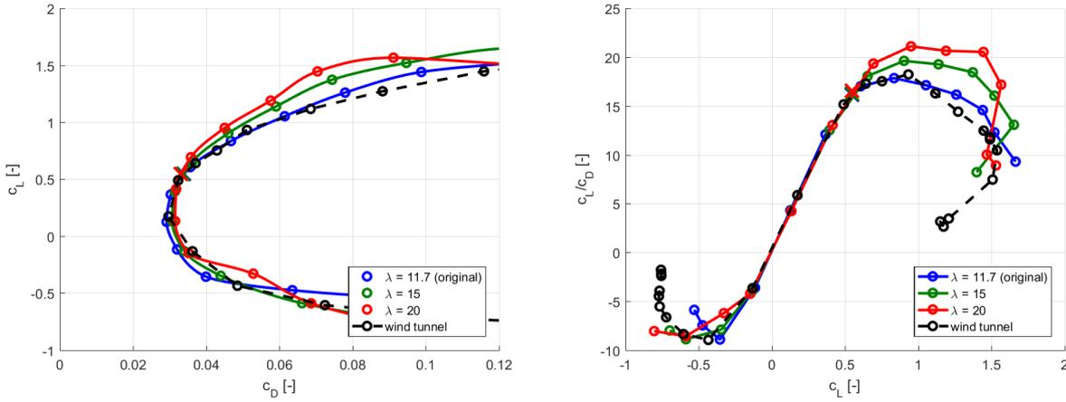
Fig. 4: Aerodynamic polar and lift to drag ratio for three different wing aspect ratio geometry.
