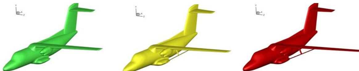
*Fig. 1: Methods Computed variants of the L-610. The green colored model is the original airplane. Yellow colored is the new one with the strut and the aspect ratio of 15. The red one is the new model with the strut and the aspect ratio of 20.*
