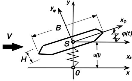
Fig. 1: Schematic 2DOF model of a bridge girder under wind loading; the response in heave  $u(t)$  (vertical direction) and pitch  $\varphi(t)$  (rotation around point S) is assumed.
