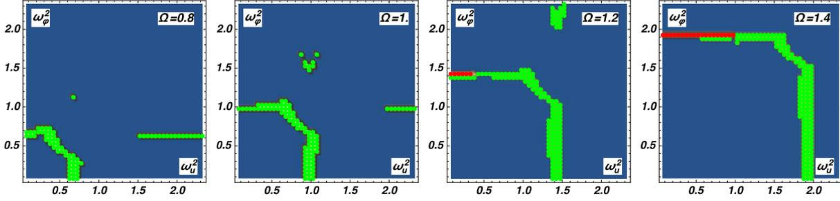
Fig. 2: Number of solutions in the  $\omega_u^2 \times \omega_\phi^2$  plane: blue – unique, green dots – threefold, red dots – fivefold solutions (excitation in the direction  $u$  only).
