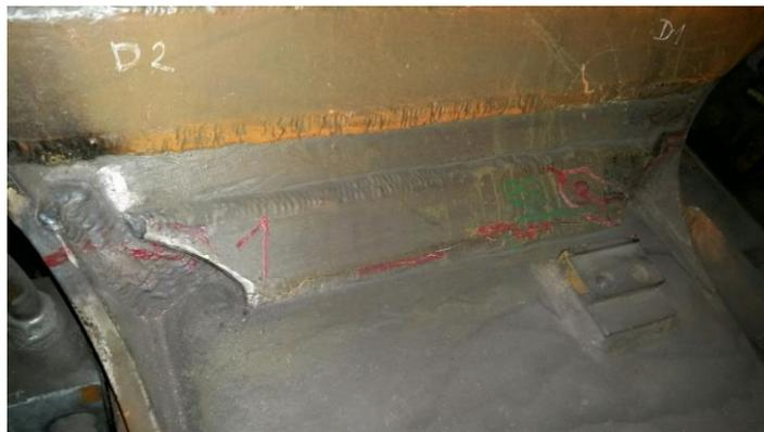
*Fig. 4: One of the detected cracks.*
