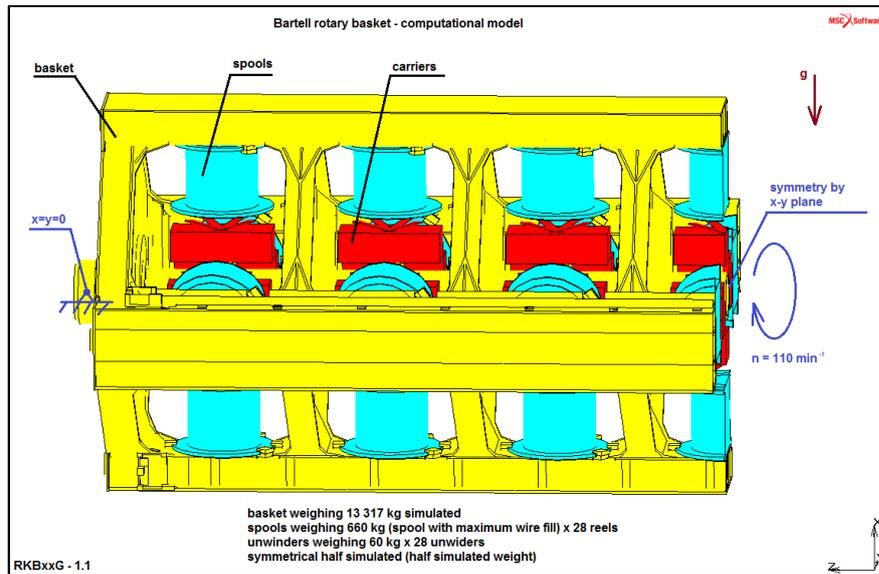
Fig. 2: Computational model for elasticity and strength analysis by ŽĐAS, a. s.
