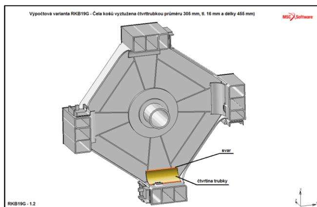
Fig. 3: Design modification proposed by ŽĎAS, a. s.
