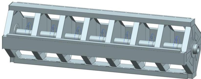
*Fig. 1: Assembly of one rotary basket.*
