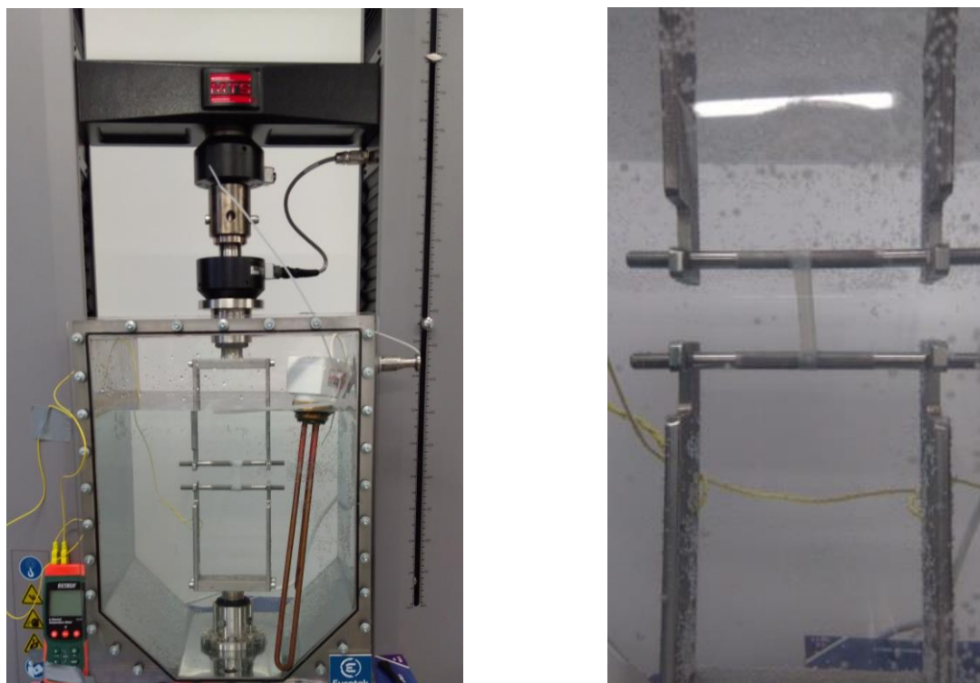
Fig. 2: Photographs of specimen, mounted in specially designed grips, immersed in a physiological chamber.
