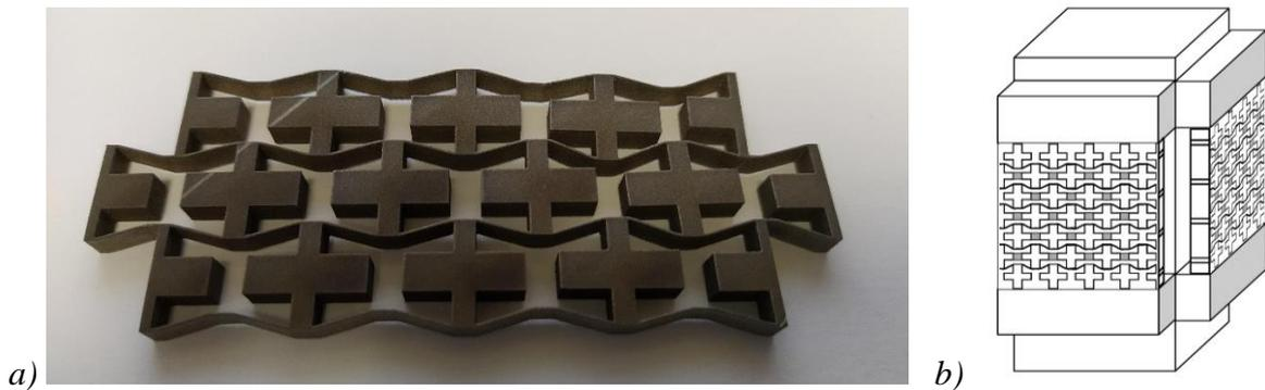
Fig. 2: Prototype of stain steel structure and proposed metamaterial application.
