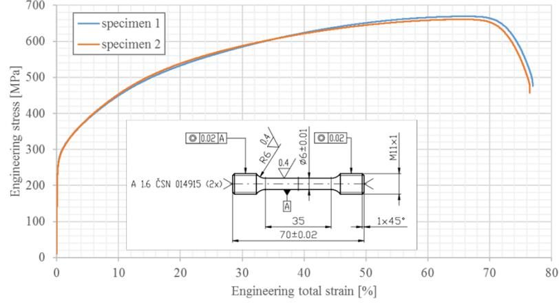
Fig. 1: Test specimen geometry, and measured stress-strain relation.
