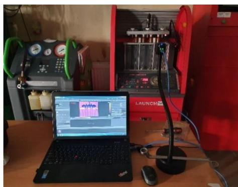
The test stand was equipped with petrol injectors from a Nissan X-trail vehicle used in 2500 cc engines, while the test stand was equipped with a FLIR AX5 camera for continuous thermal imaging measurements.
