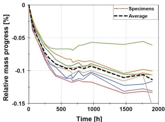
Fig. 2: Relative mass progress of specimens.
