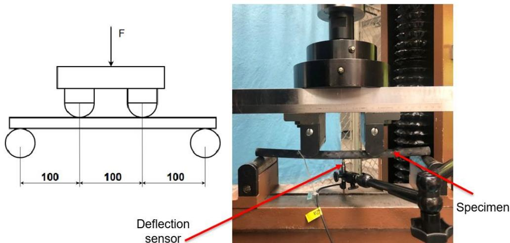
Fig. 1: 4-point bending setup.
