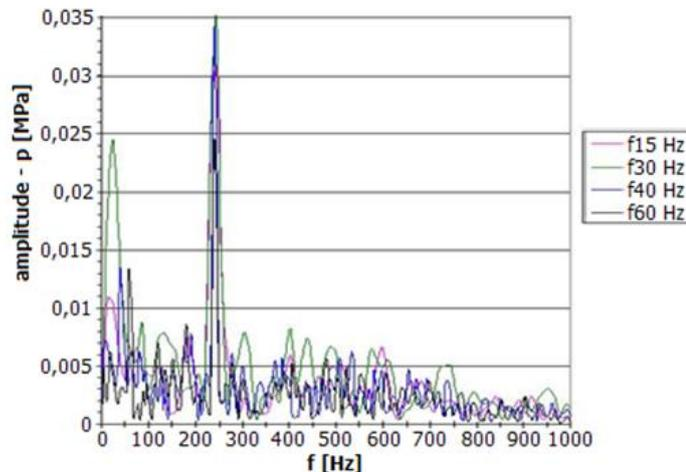
Fig. 1: Amplitude-frequency spectrum of pressure pulsation in hydraulic system with conventionally electrically controlled single-stage slide valve forced with frequency  $f = 15, 30, 40$  and  $60$  Hz. Mean pressure 2 MPa, mean flow rate  $6.5 \text{ dm}^3/\text{min}$ .
