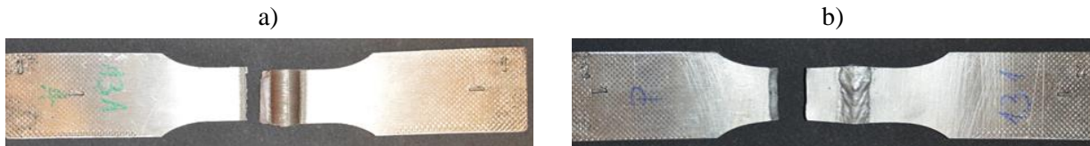
Fig. 3: Form of damage to welded joints samples made using the method: a) 131 mechanized; b) 131 semi-automatic.
