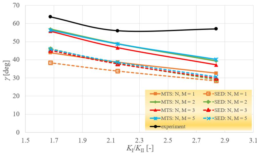
Fig. 2: Dependence of the crack deflection angle on the mixed-mode ratio for the critical distance  $r_c = 0.5$  mm: comparison between experiment and multi-parameter MTS and SED criterion considering 1, 2, 3 and 5 initial terms of the WE.
