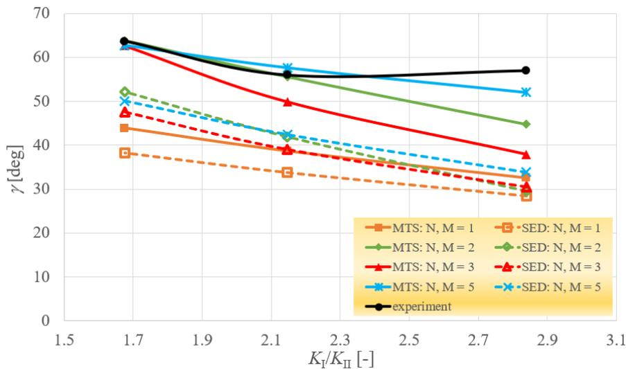
Fig. 3: Dependence of the crack deflection angle on the mixed-mode ratio for the critical distance  $r_c = 1.5$  mm: comparison between experiment and multi-parameter MTS and SED criterion considering 1, 2, 3 and 5 initial terms of the WE.
