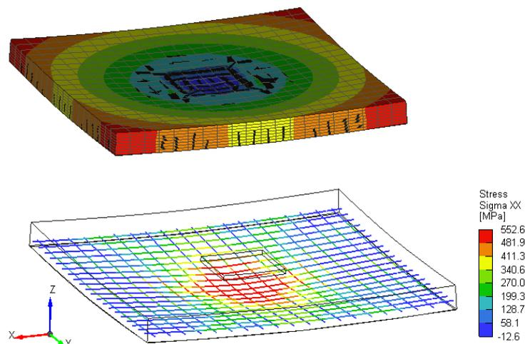
Fig. 3: RC slab with crack and reinforcement.
