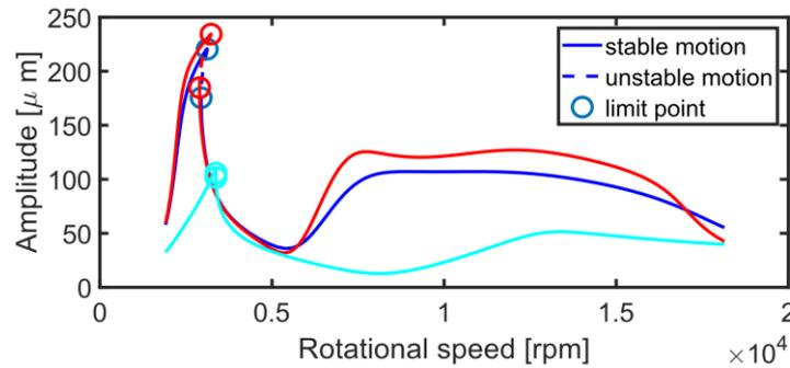
Fig. 5: Amplitude-frequency response of the rotor system with SFDs. The color of the curve represents model with variations of the damper clearance and the damper length: the blue curve (250  $\mu\text{m}$ , 22 mm), the red curve (250  $\mu\text{m}$ , 18 mm), and the cyan curve (125  $\mu\text{m}$ , 22 mm). The amplitude represents eccentricity maximum.
