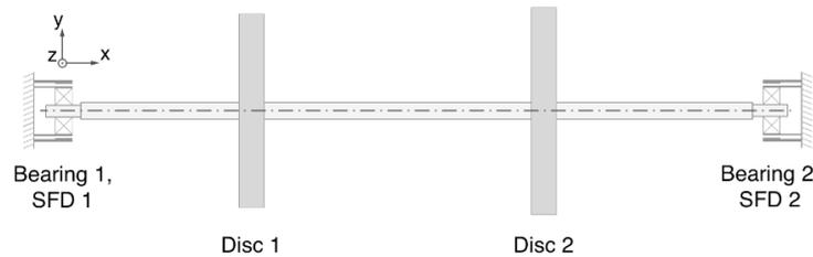
Fig. 4: Scheme of the rotor system with SFDs.
