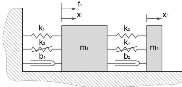
Fig. 1: Scheme of the two DOF oscillator with cubic springs.
