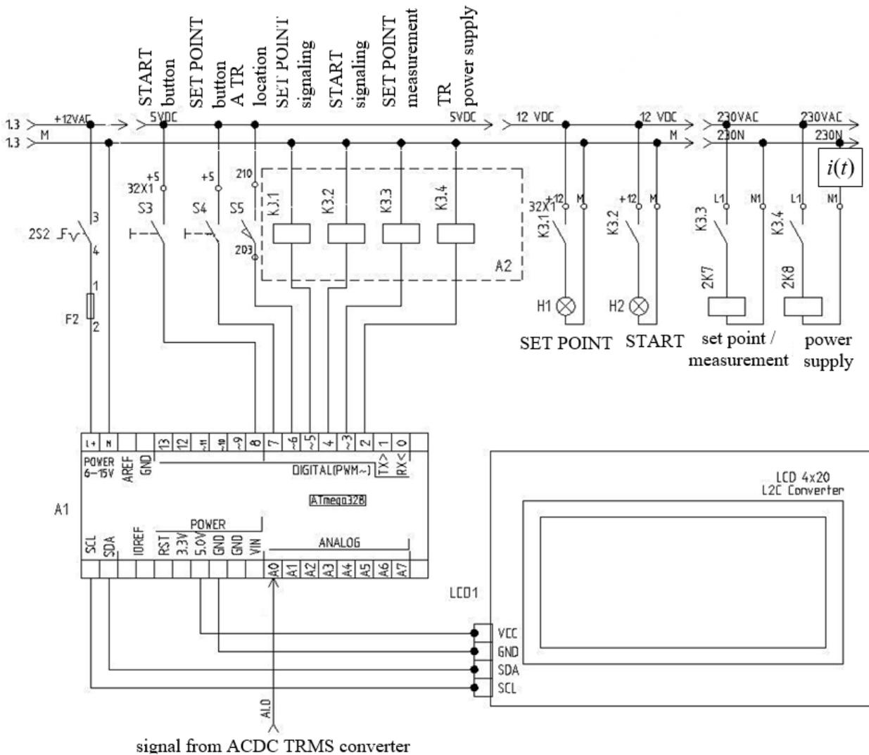
Fig. 3: Control system diagram.
