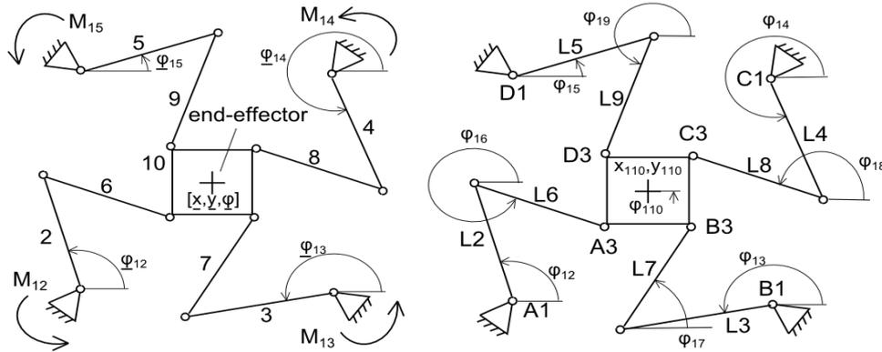
Fig. 2: Mechanism 4RRR with kinematic model (“Crosshead”).
