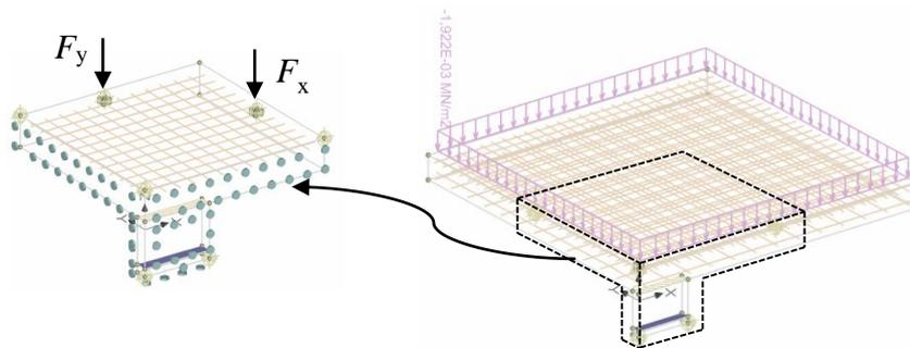
Fig. 3: a) Loading conditions of isolated and continuous flat slab.
