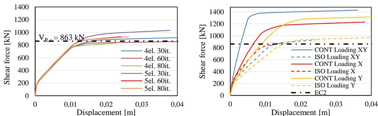
Fig. 4: a) The dependence of the increasing force on displacement measured on isolated models; b) the comparison of the dependence of the increasing force on displacement between isolated and self-confined models.
