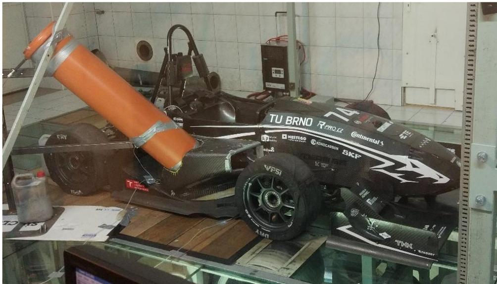
*Fig. 1: Dragon 8 in wind tunnel.*
