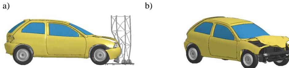
*Fig. 3: Numerical model: a) during the crash; b) final state.*
