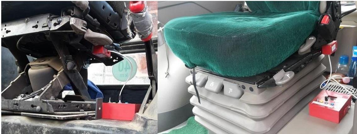
Fig. 2: Measurement of vibrations in real conditions.
