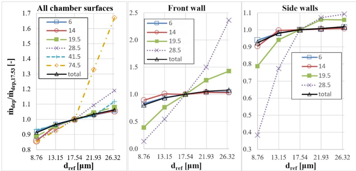
Fig. 2: Dependence of deposition flows of individual particle size fractions on reference diameter value.
