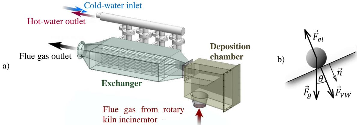
Fig. 1: a) Flue gas system scheme; b) forces considered in model of (Wacławiak and Kalisz, 2012).
