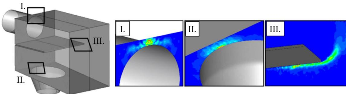
Fig. 3: Locations with high values of mass deposition flux for  $d_{ref} = 17.53 \mu\text{m}$ . Highest values are (I. – front wall)  $2.29 \cdot 10^{-2}$ , (II. - bottom)  $3.85 \cdot 10^{-3}$  and (III. – side wall)  $5.67 \cdot 10^{-3} \text{ kg} \cdot \text{s}^{-1} \cdot \text{m}^{-2}$ .
