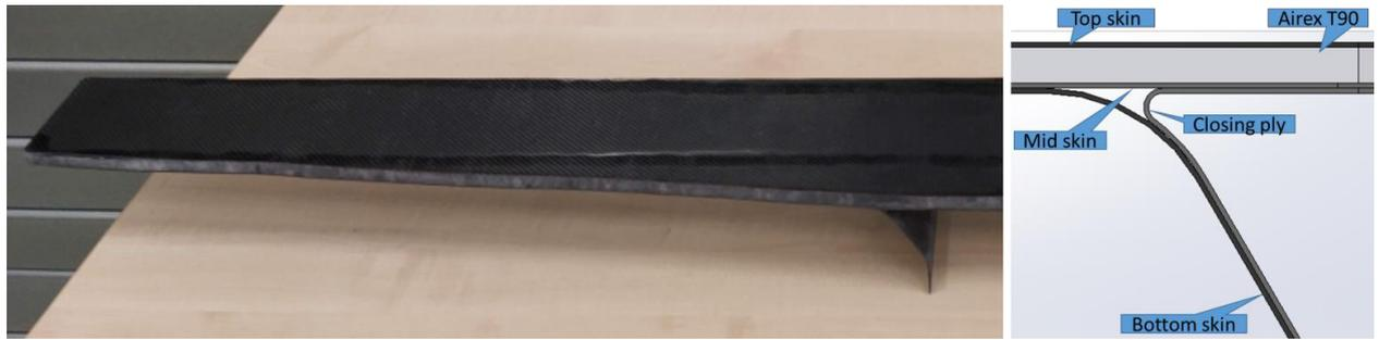
Fig. 1: Left half of fabricated empennage model from carbon fiber laminate and detail of co-cured parts.
