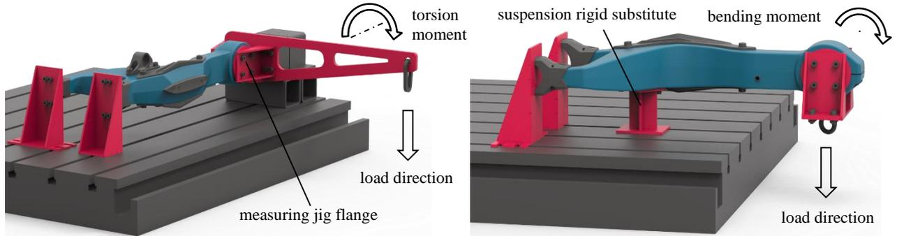
Fig. 1: Measuring setup: a) torsional stiffness measuring; b) vertical stiffness measuring.
