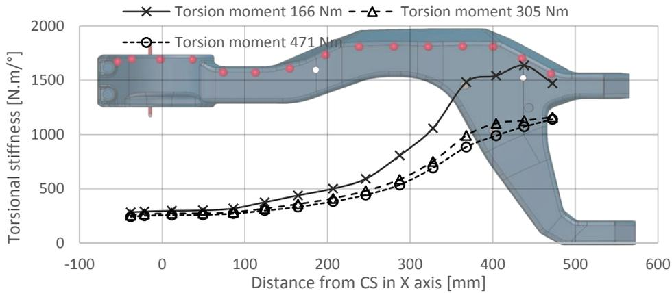
Fig. 2: Torsional stiffness distribution over the length of the swingarm.
