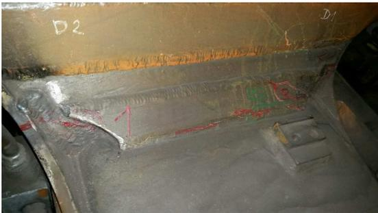
Fig. 4: One of the detected cracks
