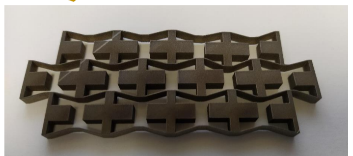
Prototype of stain steel auxetic structure
