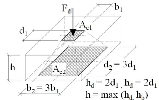
Fig. 3: Design distribution areas for determination of bearing resistance force (EN 1992-1-1).
