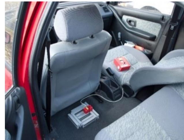
IMU location in the vehicle
