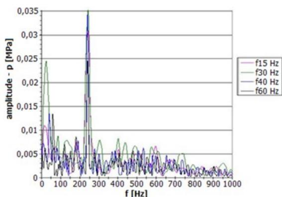
Fig. 1. Amplitude-frequency spectrum of pressure pulsation in hydraulic system with conventionally electrically controlled single-stage slide valve forced with frequency  $f = 15, 30, 40$  and  $60$  Hz. Mean pressure  $2$  MPa, mean flow rate  $6.5$  dm<sup>3</sup>/min.
