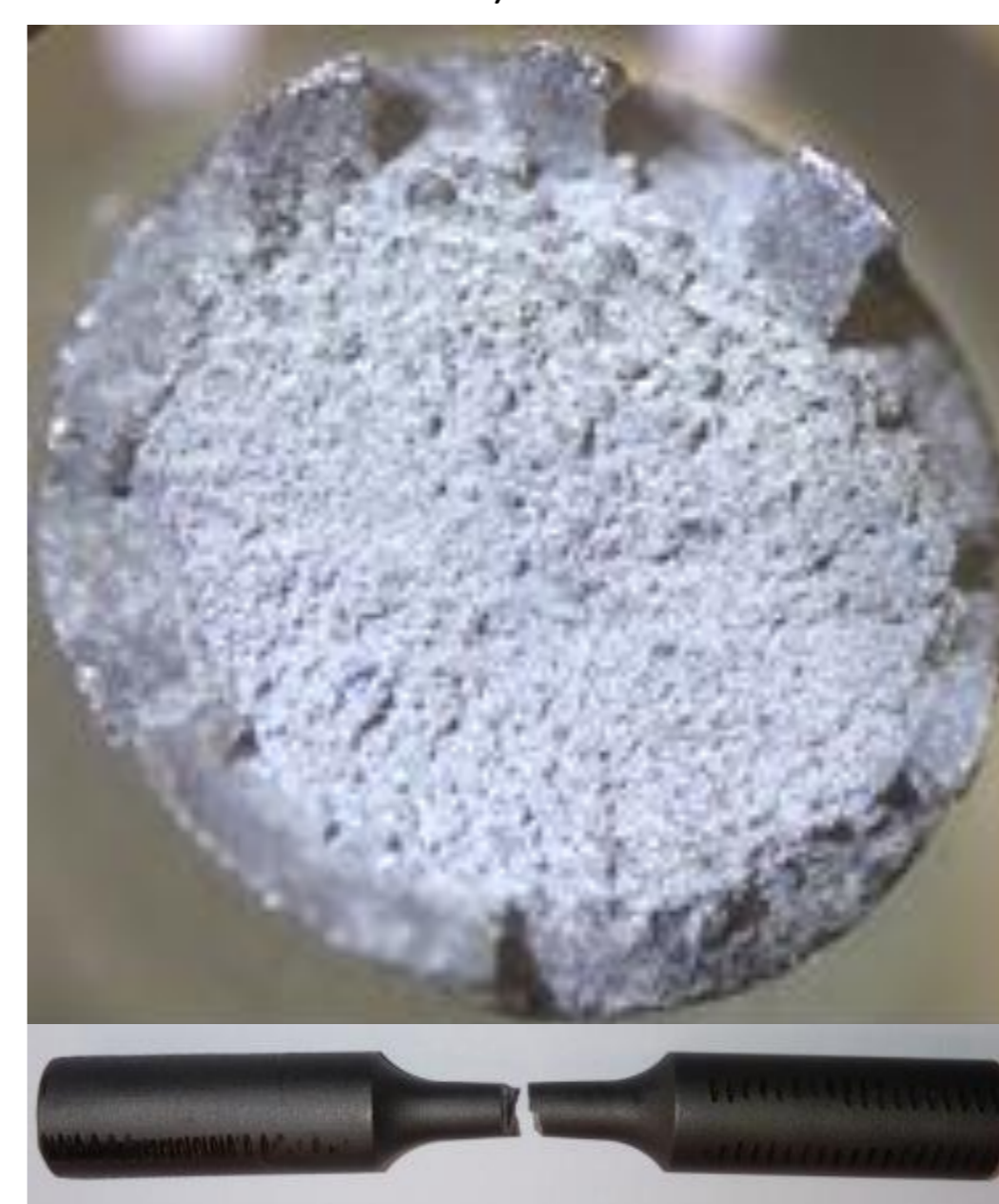
Fig. 5. Microscopic photos of fractures of samples after rupture: a - additive DMLS technology, b - from a drawn bar with a diameter of 12 mm (turned samples)
