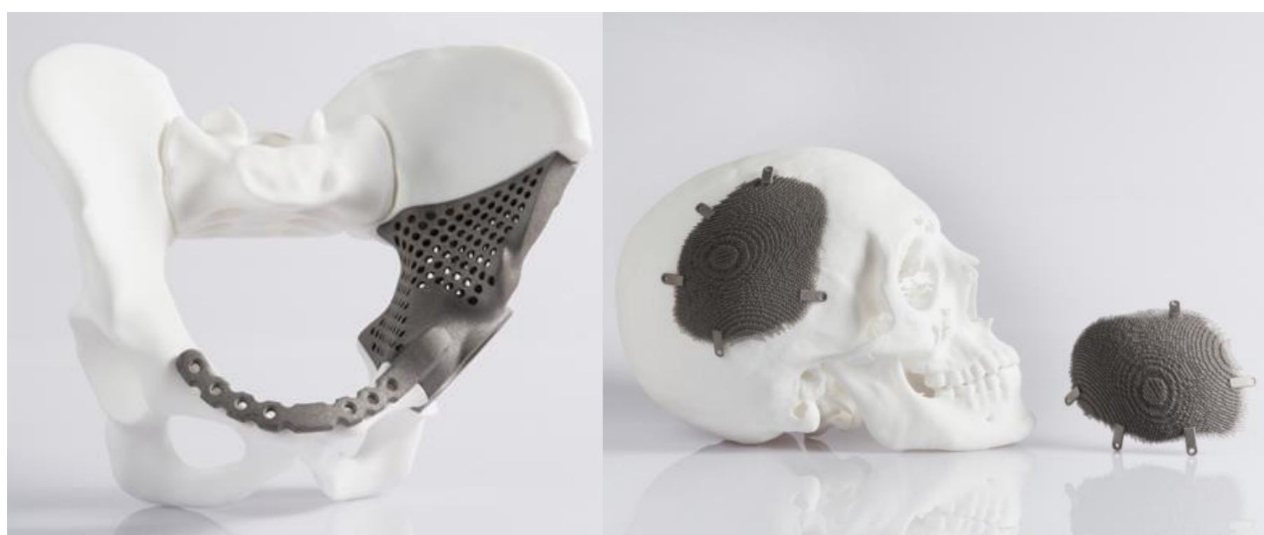
Fig. 1. Implants made in DMLS technology ( www.eos.info )
