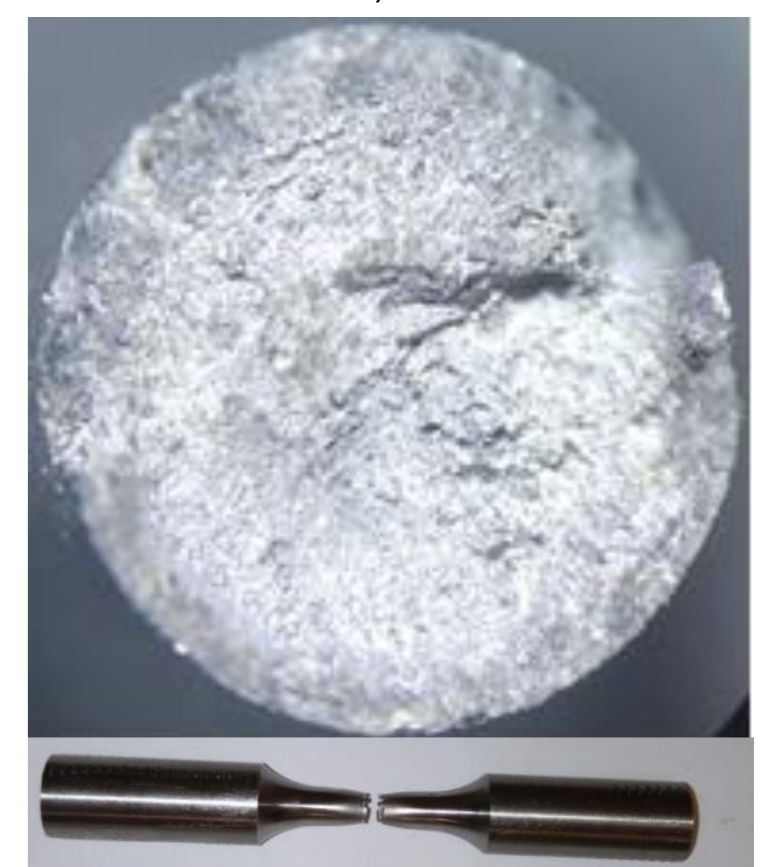
Fig. 5. Microscopic photos of fractures of samples after rupture: a - additive DMLS technology, b - from a drawn bar with a diameter of 12 mm (turned samples)
