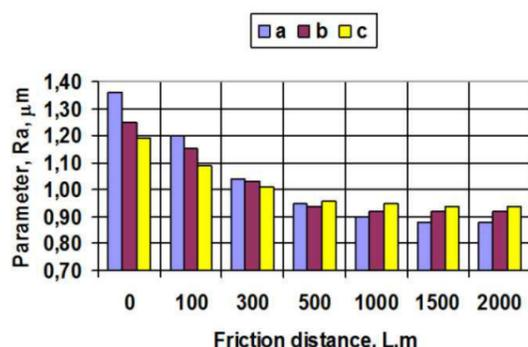
Fig. 3. The values of roughness parameter Ra as a function of friction path for surfaces after honing and for the following angles of marks after treatment: a) α = 0°; b) α = 45°; c) α = 180°
