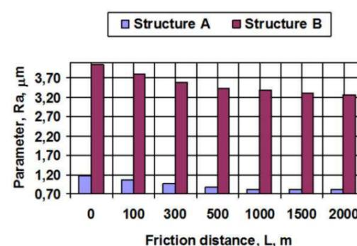
Fig. 4. Surface roughness Ra parameter value as a function of friction path for surfaces after electrical discharge machining
