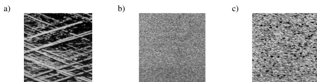
Fig. 1. Surface structure after erosive treatment: a) after electrochemical abrasive honing, b) after electro-erosion treatment at 1 A discharge current and 3.2 μs discharge time, c) after electro-erosion treatment at 6 A discharge current and 100 μs discharge time
