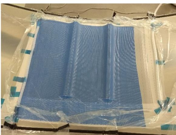
Fig. 2. Manufacturing of the panel – vacuum infusion process
