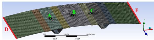
Fig. 3. FE model of the panel and boundary conditions
